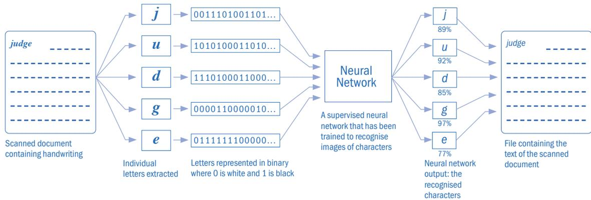
Figure 4 Using a neural network to identify handwriting
